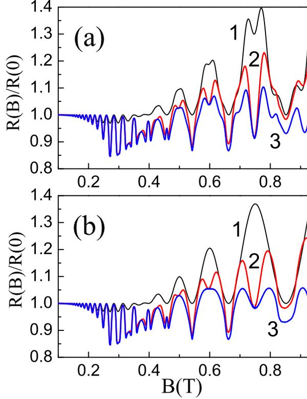
FIG. 7: (Color online) (a) Calculated magnetoresistance of the sample B at  $T = 4.2$  K and  $I = 120$   $\mu$ A. The plot 1 correspond to simple theory [Eq. (16)], while the others represent the results of numerical solution of Eq. (14) for the cases of subband-independent electron-electron scattering (2) and only intrasubband electron-electron scattering (3). (b) The same plots, where the SdHO contribution is excluded. The density of states is found within the SCBA.
