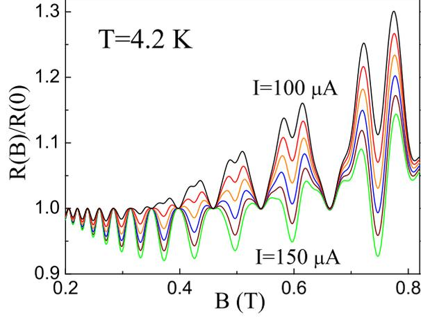
FIG. 9: (Color online) Evolution of the nonlinear magnetoresistance calculated using the parameters of the sample B when the current varies from 100 to 150  $\mu\text{A}$  with the step of 10  $\mu\text{A}$ . The Gaussian model of the density of states and the assumption of subband-independent electron-electron scattering are used.
