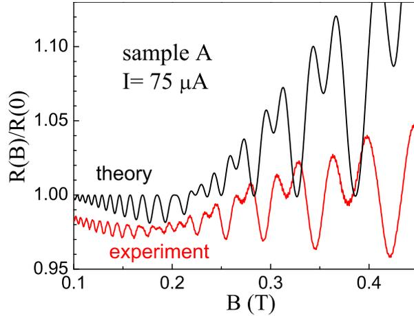
FIG. 10: (Color online) Comparison of the measured and calculated nonlinear magnetoresistance in the sample A at  $T = 4.2 \text{ K}$  and  $I = 75 \mu\text{A}$ . The Gaussian model of the density of states and the assumption of subband-independent electron-electron scattering are used in the calculations.
