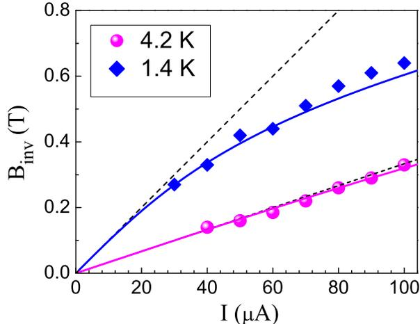
FIG. 5: (Color online) Dependence of the inversion field on the current for the sample B at  $T = 4.2$  K and  $T = 1.4$  K. (points) The dashed lines correspond to a linear  $B_{\text{inv}}(I)$  dependence assuming  $\tau_{in} = 64$  ps at 4.2 K (580 ps at 1.4 K). The solid lines represent the calculated  $B_{\text{inv}}(I)$  dependence taking into account electron heating by the current.
