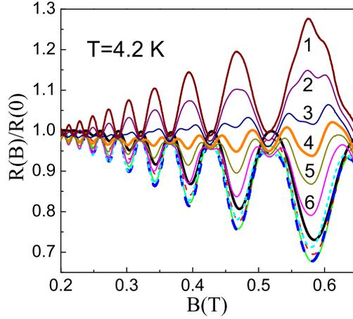
FIG. 4: (Color online) Magnetoresistance of the sample B at  $T = 4.2$  K. The values of the current ( $\mu\text{A}$ ) are 1, 50, 80, 100, 120, and 150 for the curves marked by the numbers from 1 to 6, respectively. The other curves corresponds to the currents of 200 (short dash), 250 (bold dash) 300 (solid), 350 (dash), and 400 (bold)  $\mu\text{A}$ .
