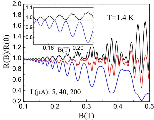
FIG. 1: (Color online) Magnetoresistance of the sample A for three different currents  $I$  at  $T = 1.4$  K. The oscillations are inverted with the increase of the current. The inset shows the linear and non-linear (at  $I = 200 \mu\text{A}$ ) magnetoresistance in the low-field region.
