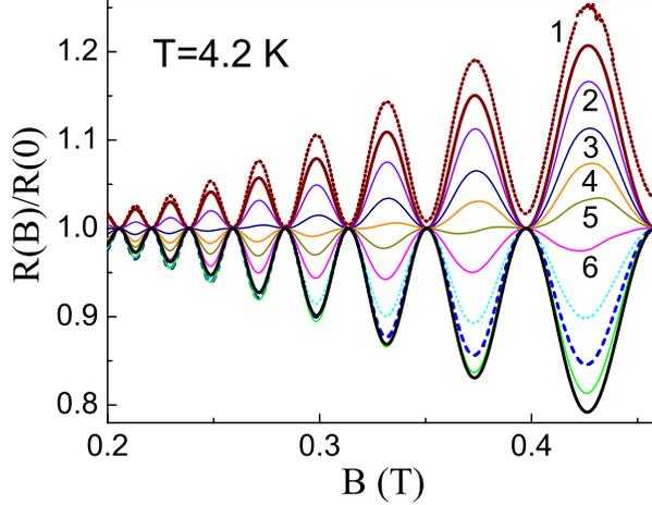
FIG. 6: (Color online) Calculated magnetoresistance of the sample B at  $T = 4.2$  K and different currents: 1, 50, 80, 100, 120, and 150  $\mu\text{A}$  for the curves marked by the numbers from 1 to 6; the other curves corresponds to  $I = 200$  (short dash), 250 (bold dash), 300 (solid), and 400 (bold)  $\mu\text{A}$ . The additional (dashed) line 1 shows the linear magnetoresistance determined by the SCBA calculation of the density of states in Eq. (13).
