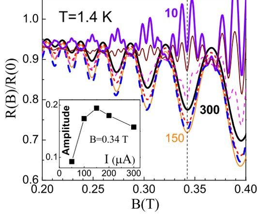
FIG. 3: (Color online) Magnetoresistance of the sample B at  $T = 1.4$  K. The values of the current are 10 (bold), 30, 50 (dash), 100 (bold dash), 150, 200 (short dash), and 300 (bold)  $\mu\text{A}$ . The inset shows amplitudes of the inverted peaks at  $B = 0.34$  T.
