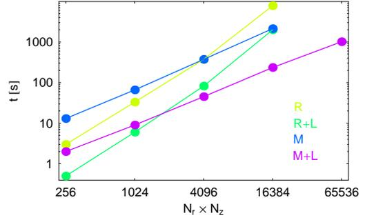
Figure 1: Execution times in seconds for different integration strategies.  $R$  denotes results obtained by iterative algorithm,  $M$  by multigrid, while  $L$  denotes multilevel prolongation method. Grids have  $N_r = N_z$ .
