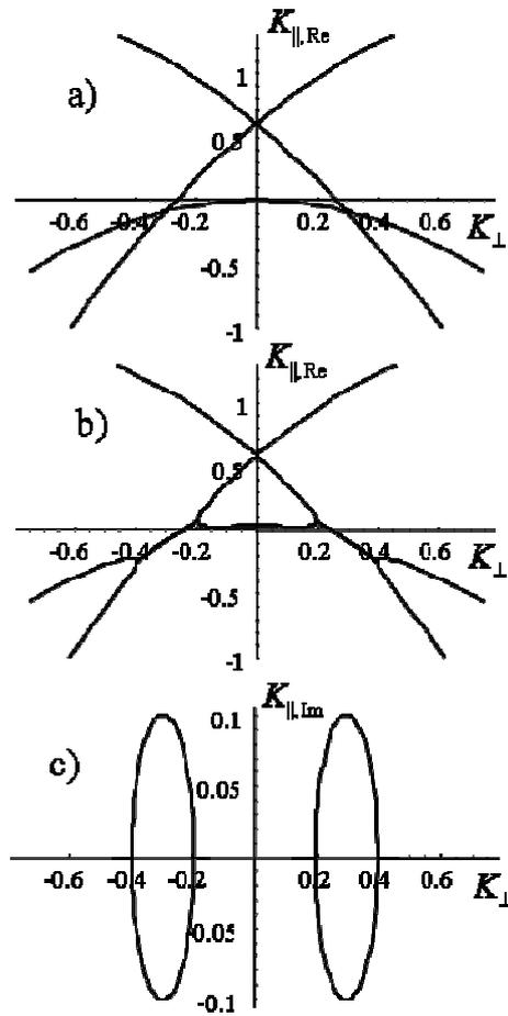
**Fig.2.** Propagation eigenvalues (real parts of  $K_{\parallel}$ ) (a,b), and growth exponents (imaginary parts of  $K_{\parallel}$ ) (c) for the three-coupled-mode model (6), in the self-collimation regime for  $Q_{\parallel} = 1.6$ . (a) illustrates the geometry of the dispersion parabolas of harmonic components with vanishing coupling ( $m \rightarrow 0$ ). (b) shows the development of a self-collimation plateau on the dispersion curves of the Bloch modes for  $m = 0.1$ .
