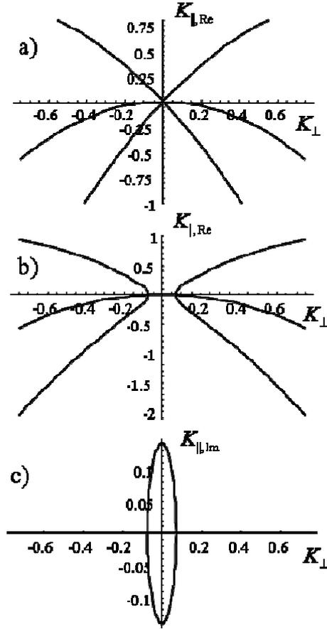
**Fig.4.** The propagation eigenvalues (real parts of  $K_{\parallel}$ ) (a,b), and the growth exponents (imaginary parts of  $K_{\parallel}$ ) (c), for the three-coupled-mode model (6), in the spatial filtering regime. (a) Geometry of dispersion parabolas of harmonic components. (b) Plateau of mode-locking for  $m = 0.1$  (c) Angular gain profile.  $Q_{\parallel} = 1.0$
