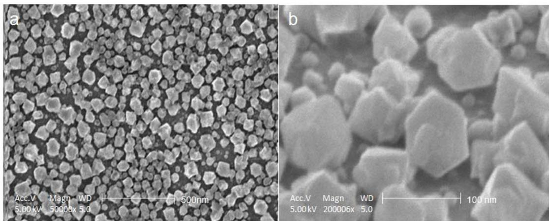
**Figure 1:** FE-SEM image of non-uniform shaped nanoparticles synthesized at 950 °C, on the Si (100) surface. (a) Top view of the nanoparticles. (b) A high magnification image at a viewing angle of 45°.
