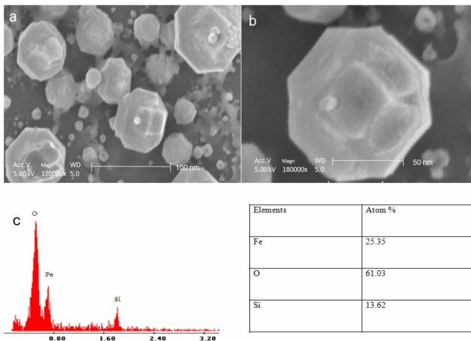
Figure 2: FE-SEM image of the  $\text{Fe}_2\text{O}_3$  polyhedral nanocrystals obtained at  $1000\text{ }^\circ\text{C}$  annealing temperature. (a) The nanocrystals are polyhedral with different smooth surfaces. (b) High resolution FE-SEM image clearly indicating different faces of polyhedral nanocrystal. (c) Represents the EDX spectrum with atomic percentage in table.
