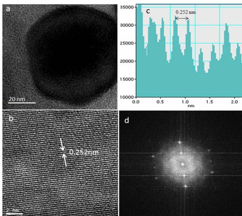
Figure 3: (a) TEM image, a  $\text{Fe}_2\text{O}_3$  polyhedral nanocrystal. (b) High resolution TEM image showing parallel 110 planes. (c) Atomic profile for the HRTEM image. (d) Selected area diffraction pattern (SADP) of the nanocrystal.
