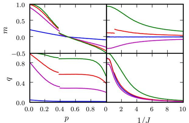
FIG. 4: (Color online) Magnetization  $m$  and spin-glass order parameter  $q$  for the Ising spin glass on an Apollonian network. In the left panels, the curves, consecutively left-most from the top, are for constant temperature  $1/J = 0.2, 1.0, 2.0, 10.0$ . In the right panels, the curves, consecutively from the top, are for antiferromagnetic bond concentration  $p = 0.10, 0.38, 0.50, 0.90$ .
