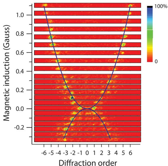
FIG. 3: High order quasi-Bragg diffraction as a function of applied magnetic field. The spin polarized beam was prepared in the  $|M = 1\rangle$  state with zero transverse momentum. As the magnetic field is stepwise increased, the detected diffraction patterns for atoms in the  $|M = -1\rangle$  output state are displayed. The double parabola (solid line) indicates where the magnetic energy balances the gain in kinetic energy.
