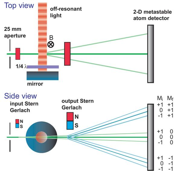
FIG. 2: Double Stern Gerlach deflection ‘tags’ each atom according to its initial and final magnetic substate. Diffraction patterns emerge horizontally, perpendicular to the magnetic deflection.
