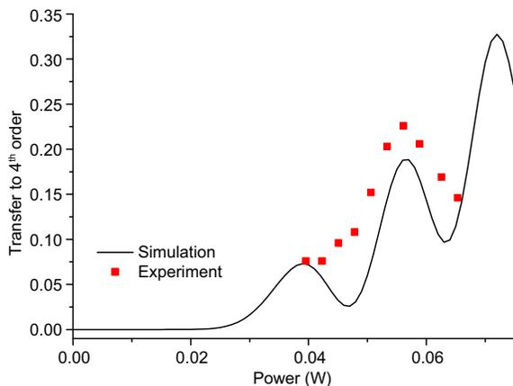
FIG. 5: Efficiency of 4<sup>th</sup> order  $|M = 1\rangle$  to  $|M = 0\rangle$  quasi-Bragg diffraction versus laser power.
