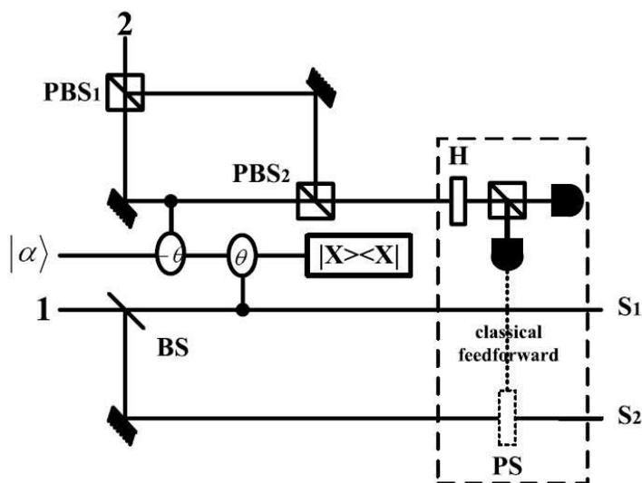
FIG. 1: Controlled-path gate with weak cross-Kerr nonlinearity. This gate is implemented with the probability  $1/2$ . If the setups in the dashed line are used, this gate can be used to realize all possible bipartite positive-operator-value measurements of two-photon polarization states with the probability  $1/2$ .
