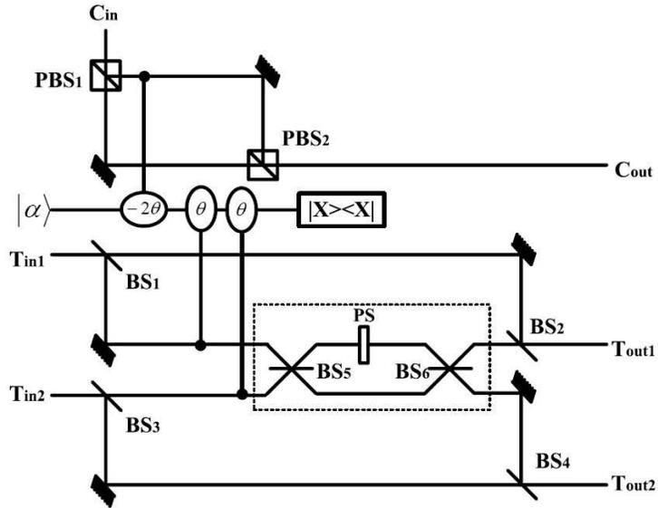
FIG. 3: Fredkin gate with the weak cross-Kerr nonlinearities. The setups in the dashed line will complete the transformation  $|\Psi^-\rangle \rightarrow -|\Psi^-\rangle; |\Psi^+\rangle (|\Phi^\pm\rangle) \rightarrow |\Psi^+\rangle (|\Phi^\pm\rangle)$ . Associated with the nonlinearities and appropriate transmissivities of four beam splitters, the Fredkin gate is realized with the probability  $1/16$ .
