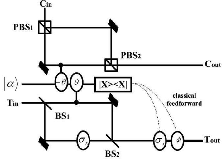
FIG. 2: CNOT gate with the weak cross-Kerr nonlinearity. Assisted by a classical feedforward, this gate can be implemented with the probability  $1/2$ .
