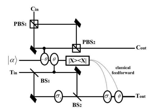
FIG. 2: CNOT gate with the weak corss-Kerr nonlinearity. Assisted by a classical feedforward, this gate can be implemented with the probability 1/2.
