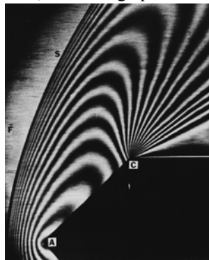
Fig. 3. [1, ph. 234]. Interferogram, lines of constant density, M = 2.5 . Supersonic foregoing shock wave and subsonic area between it and the body. See Fig. 2.
