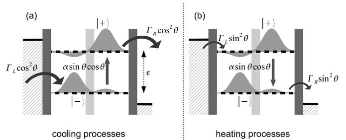
FIG. 3: Dominant cooling (a) and heating (b) processes in the parameter region of optimal cooling in Fig. 2. States  $|-\rangle$  and  $|+\rangle$  denote the bonding and antibonding states at frequency difference  $\epsilon = \sqrt{\Delta^2 + 4T_c^2}$ . The rates are reported in the new basis, with  $\tan \theta = 2T_c/(\Delta + \epsilon)$ . For  $\Delta > 0$ , then  $\tan^2 \theta < 1$  and the processes in (a) are faster, so that the resonator is cooled.
