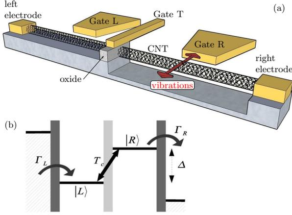
FIG. 1: (a) Sketch of the double quantum dot, carbon-nanotube (CNT) device. The dot on the right is suspended, and mechanically oscillates. (b) The single-electron levels  $|L\rangle$  and  $|R\rangle$ , at (tunable) frequency difference  $\Delta$ , are coherently coupled with tunneling rate  $T_c$ . Left (right) electrode acts as electron source (drain) at rate  $\Gamma_L$  ( $\Gamma_R$ ). By suitably tuning the parameters the oscillator can be cooled to the ground state.
