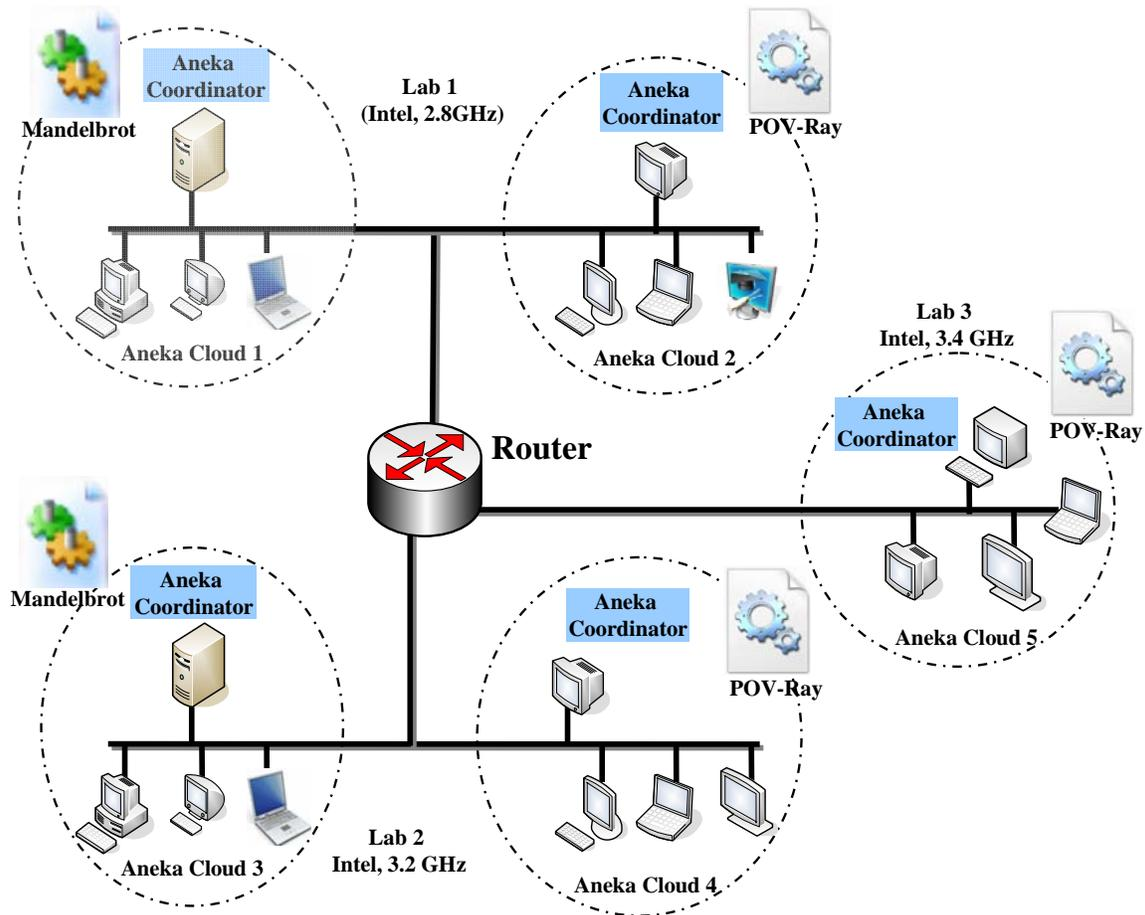
Figure 11: Aneka-Federation test bed distributed over 3 departmental laboratories.
