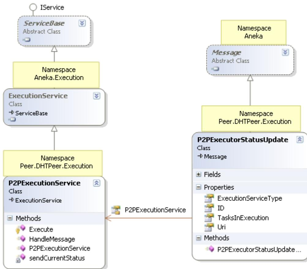
Figure 6: Class design diagram of P2PExecution service.
