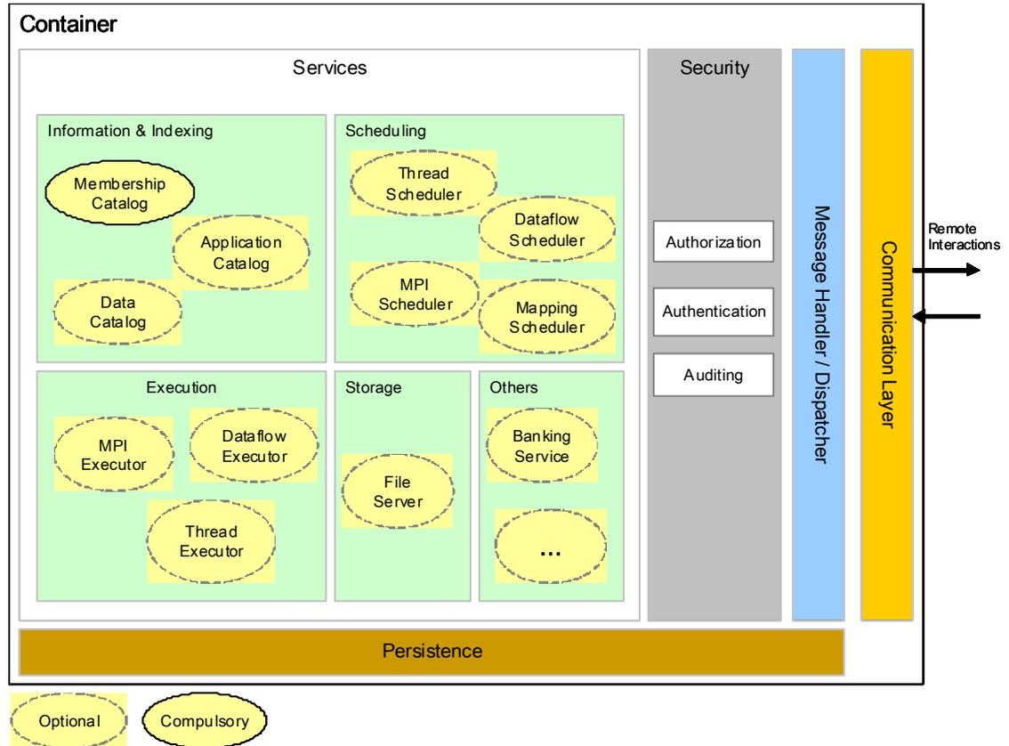
Figure 1: Design of Aneka container.
