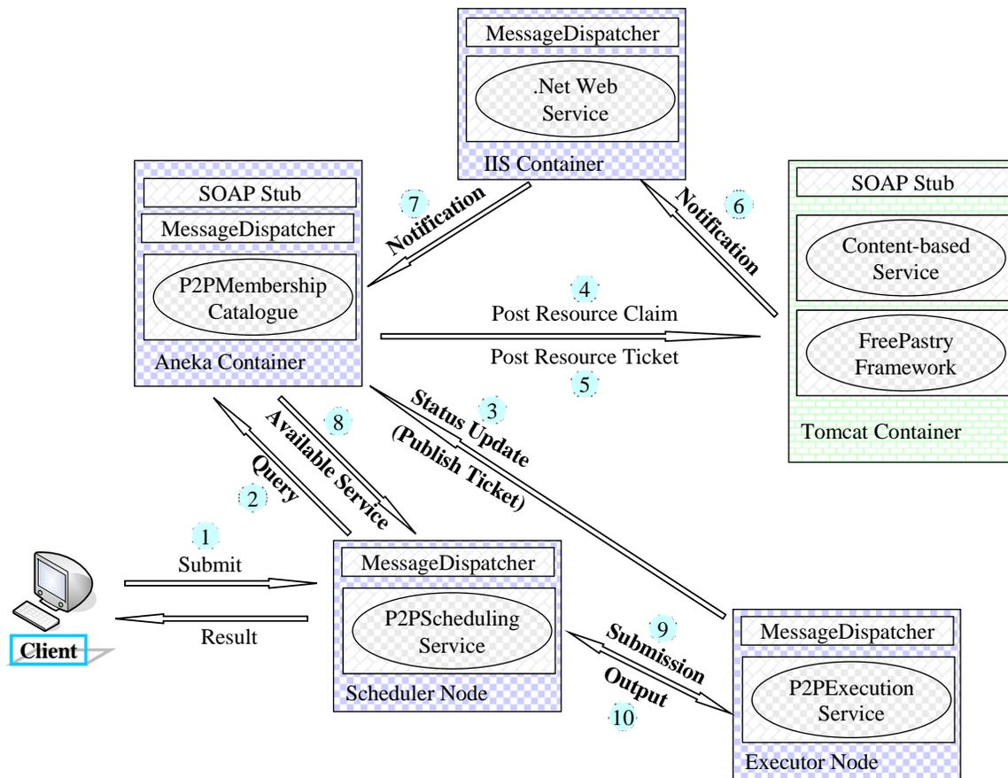
Figure 8: Application execution sequence in Aneka-Federation.
