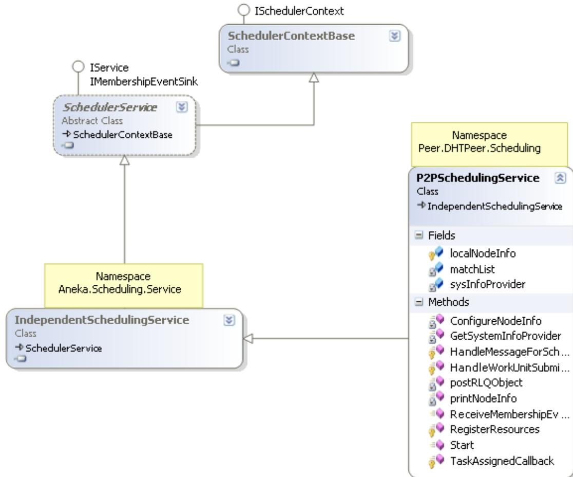
Figure 5: Class design diagram of P2PScheduling service.
