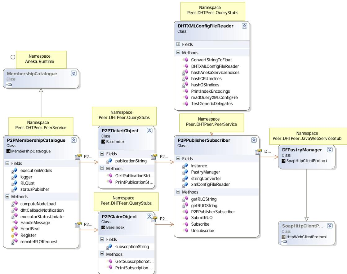
Figure 7: Class design diagram of P2PMembershipCatalogue service.
