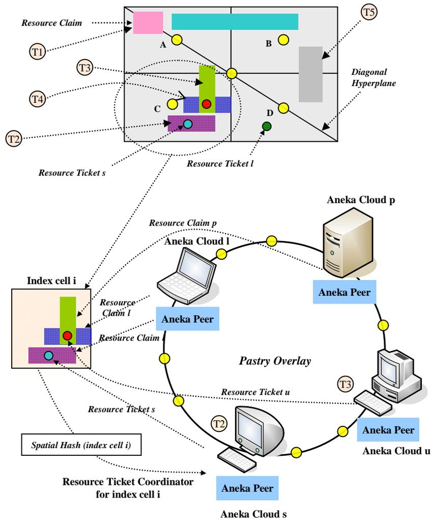
Figure 10: Resource claim and ticket object mapping and coordinated scheduling across Aneka Enterprise Cloud sites. Spatial resource claims  $\{T1, T2, T3, T4\}$ , index cell control points  $\{A, B, C, D\}$ , spatial point tickets  $\{l, s\}$  and some of the spatial hashings to the Pastry ring, i.e. the  $d$ -dimensional (spatial) coordinate values of a cell's control point is used as the Pastry key.
