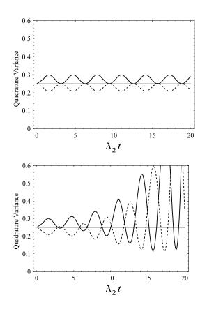
FIG. 2: Time evolution of the quadrature variances for circularly polarized modes, with  $\beta = \alpha$ ,  $Re[\alpha] = 0$  and  $Im[\alpha] = 0.3$ . (a)  $(\Delta X_+)^2$  (continuous line) and  $(\Delta Y_+)^2$  (dashed line) for  $\lambda_1/|\lambda_2| = 0$ . (b)  $(\Delta X_+)^2$  (continuous line) and  $(\Delta Y_+)^2$  (dashed line) for  $\lambda_1/|\lambda_2| = 0.1$ .
