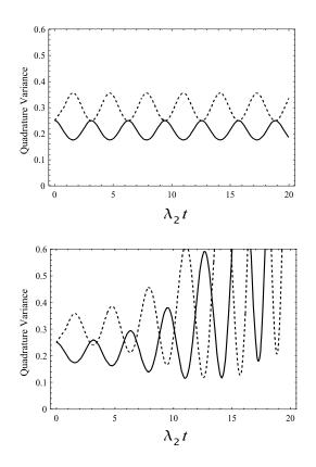
FIG. 4: Time evolution of quadrature variances for linearly polarized modes, with  $\alpha = \beta$ ,  $Re[\alpha] = 0$  and  $Im[\alpha] = 0.3$ . (a)  $(\Delta X_y)^2$  (solid line) and  $(\Delta Y_y)^2$  (dashed line) for  $\lambda_1/|\lambda_2| = 0$ . (b)  $(\Delta X_y)^2$  (solid line) and  $(\Delta Y_y)^2$  (dashed line) for  $\lambda_1/|\lambda_2| = 0.1$ . Mode x is left in a vacuum state.
