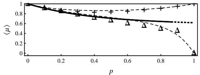
FIG. 6: Mean node value of a network using NAND and OR transfer functions from [17] and a threshold that is (+ symbols) below, and ( $\Delta$  symbols) above the intermediate fixed point defined in the text.  $p$  is the fraction of NAND nodes. Our mean field theory (dashed curves) gives a much better approximation of the dynamics than does the naive Boolean model (solid curve).
