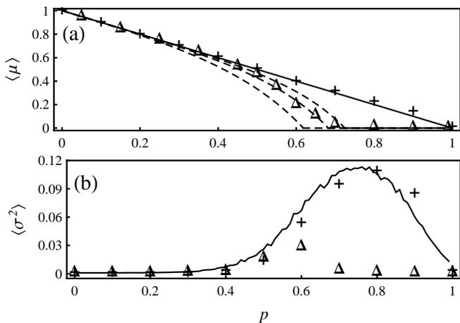
FIG. 2: (a) The mean fraction of ON nodes. The + and  $\Delta$  symbols correspond to  $S_1$  and  $S_2$ , respectively. The solid line  $\mu = 1 - p$  is the prediction for an infinite random Boolean network with a fraction  $p$  of NIF gates and  $1 - p$  of OR gates. The dashed curves show the theoretical results discussed in the text. (b) The total variance corresponding to the systems in (a). The solid curve is the average variance from simulations of the Boolean model.
