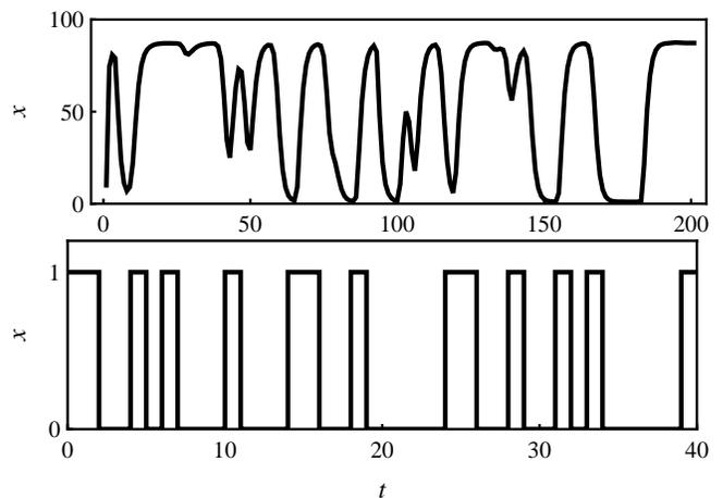
FIG. 3: Typical time series for an unfrozen node in the disordered regime ( $p = 0.8$ ) in a continuous system,  $S_1$ , and in a synchronously updated Boolean system. Both systems have attractors with complex dynamics.
