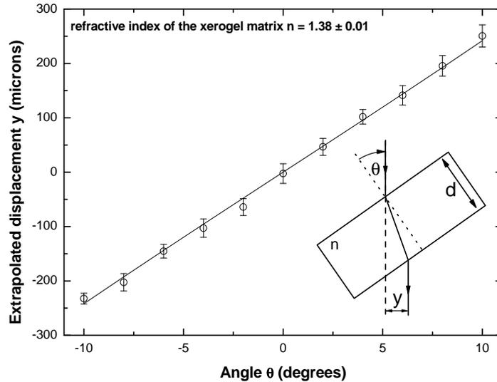
FIG. 1: Determination of the refractive index of the xerogel matrix, without PS spheres. The inset presents the setup scheme. The displacement of the back face of the sample,  $y$ , from a laser beam impinging on the front face, is monitored as a function of incident angle  $\theta$ . Simple geometric optics allows the measurement of the matrix refractive index as  $1.38 \pm 0.01$ . Knowing the refractive index of the matrix is a key characterization of the diffusive samples.
