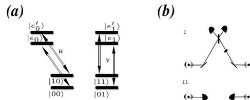
FIG. 4: (a) to fight photon losses the atom needs to store a second qubit to carry a security copy of the photon. (b) in the first attempt we try to establish an evolution by sending the photons on a beam-splitter. In case of success we erase the security copy, in case of failure we can reuse the copy by measuring in different basis.
