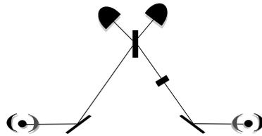
FIG. 2: Two distance atoms are effectively coupled by sending photons coming out of the cavity to a beam splitter. Depending on the measurement outcome we apply a feedback loop on the atoms until the desired evolution has been done.
