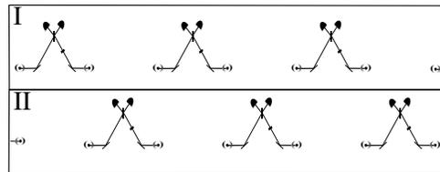
FIG. 3: To simulate a next neighbor Hamiltonian we can do  $m/2$  of the rotations in parallel. We need to basic setup such that each cavity sends a photon on a beam splitter together with either its right or its left neighbor.
