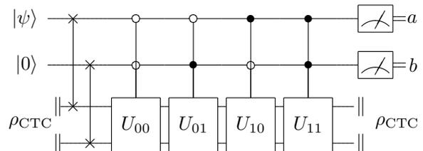
FIG. 2: The above circuit can perfectly distinguish the BB84 states  $|0\rangle, |1\rangle, |+\rangle,$  and  $|-\rangle$ . The circuit uses the standard quantum circuit notation from Ref. [11] and we define the unitaries  $U_{00}, U_{01}, U_{10},$  and  $U_{11}$  in (3).
