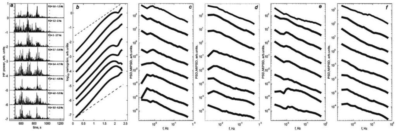
Figure 3. Limited range of self-similarity for the 2004.12.26 mega-earthquake. (*a, b, c*)– analogs of Fig 1*bcd* for SNZO, (*d, e, f*) – spectral plots only, for KONO, ALE, and ARU
