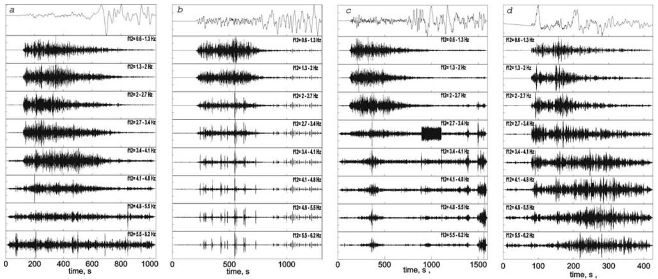
Figure 2. Examples of rejected data. (a) Event 2004.12.26 at KMBO, three lowermost traces are rejected automatically, the rest ones are qualified as usable. (b) Same event at KIV, spurious pulses of presumably instrument/digitizer origin. (c) Same event at SBA, spurious signals of unclear origin. (d) Event 1998.03.05 at WRAB. Powerful  $T$ -phase signal is seen above 3 Hz.
