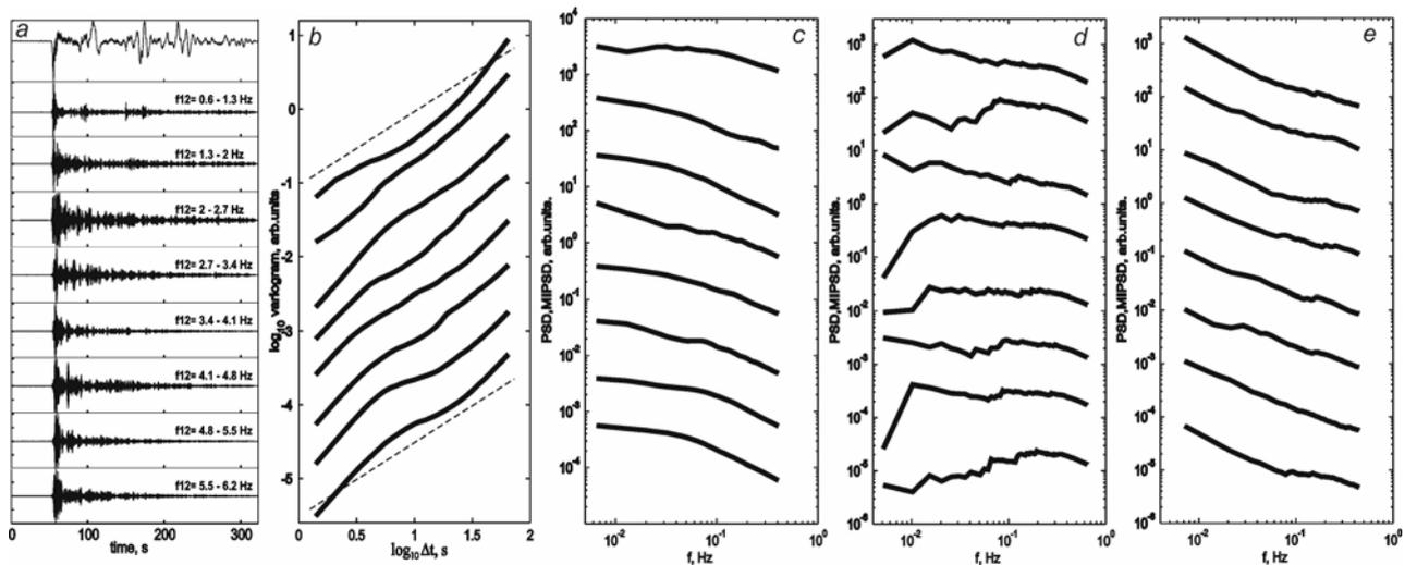
Figure 4. Examples of non-self-similar data. (*a*) bandpass-filtered traces of 150 s of the record after the first arrival of 1998.12.14 event ( $M=6.8$ ) at WRAB. (*b, c*) corresponding variograms and  $MIPSD(f)$ . (*d, e*)  $MIPSD(f)$  for 150 s of simulated stationary white noise (*d*) and for similar signal modulated by deterministic triangular envelope (*e*).
