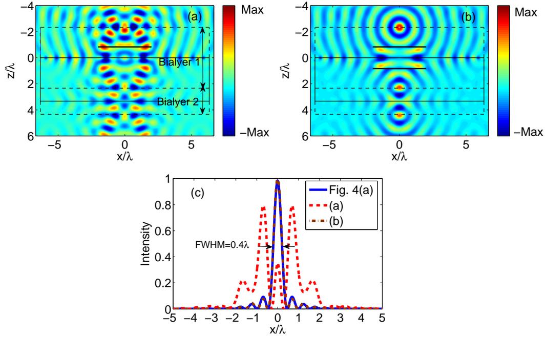
FIG. 6: Electric field distribution when (a) a current sheet  $J_s = 4A\delta(x + z/6\lambda)$   $x \in [-2\lambda, 2\lambda]$  is put in the front of the lens of Fig. 4(a); (b) the compensated current sheet is put inside the lens. (c) Field intensity at the the image plane  $z = 13/3\lambda$  for (a), (b), and also Fig. 4(a).
