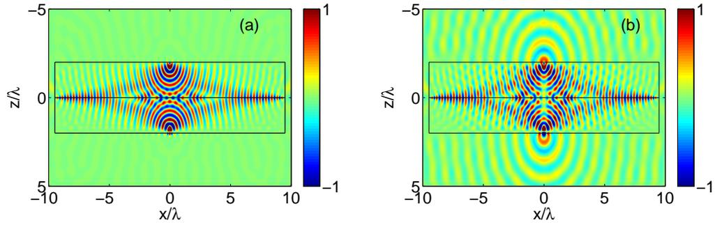
FIG. 5: Electric field distribution for (a) two current sources  $\bar{\mathcal{J}}_1 = A\delta(x)\delta(z + 1.9\lambda)\hat{y}$  and  $\bar{\mathcal{J}}_2 = -A\delta(x)\delta(z - 1.9\lambda)\hat{y}$  embedded in the bilayer ; (b) only  $\bar{\mathcal{J}}_1$  is embedded in the bilayer. The bilayer lens has the same material parameters as in Fig. 3.
