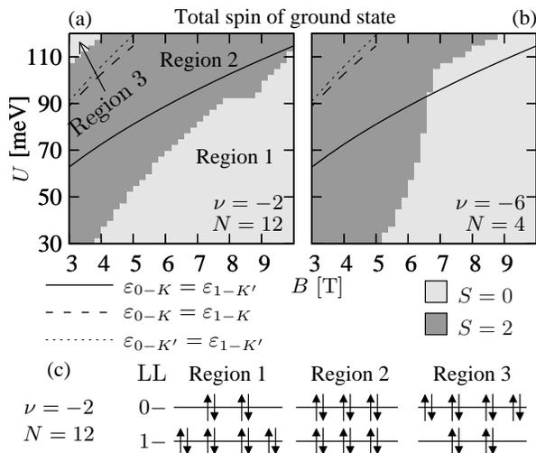
FIG. 4: The total spin of the ground state of the (a)  $\nu = -2$  and (b)  $\nu = -6$  systems.  $M = 2$  and  $N = (\nu + 8)M$ . The lines show the crossing points of the single particle states. The graining is due to the finite interval between data points. (c) The occupancy of the single electron states in the interacting many body ground state for each region of the plot in (a). The  $z$ -projection of the total spin is fixed at zero as described in the text.
