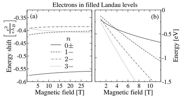
FIG. 3: (a) The energy shift per electron of filled LLs. (b) The absolute energy per electron of filled LLs showing the crossing between the  $n = 0\pm$  degenerate level and the higher LLs in the valence band. In both plots  $U = 0$ , and  $M = 5$ .
