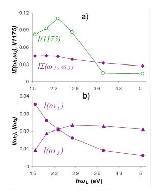
Fig. 5 a) - Evolution of relative intensities of the 1175 cm<sup>-1</sup> peak, I(1175) and *trans*-(CH)<sub>x</sub> contributions,  $I\Sigma(\omega_1, \omega_3)$  and b) relative intensities of  $\omega_1$ ,  $I(\omega_1)$  and  $\omega_3$ ,  $I(\omega_3)$  peaks as a function of the laser excitation energy  $\hbar\omega_L$ .
