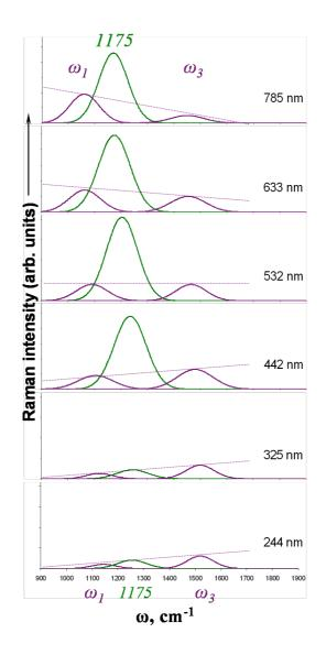
Fig. 4 - Changes in the fitted  $\omega_1$ ,  $\omega_3$  and  $I175 \text{ cm}^{-1}$  bands (intensity magnified by a factor of 5) relative to the laser excitation energy  $\hbar\omega_L$  in the spectra of *a*-C:H. Light dotted line over  $\omega_1$  and  $\omega_3$  bands denotes the  $I(\omega_3)/I(\omega_1)$  trend.
