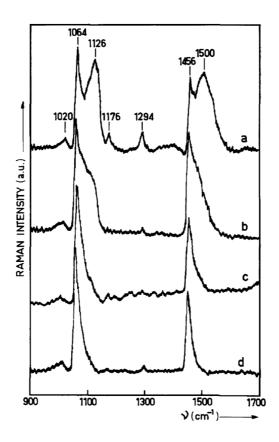
Fig. 1 - Resonant Raman spectra of bulk *trans*-(CH)<sub>x</sub> at 78 K taken for different laser excitation wavelengths. a)  $\omega_L = 457.9$  nm; b)  $\omega_L = 514.5$  nm; c)  $\omega_L = 600$  nm; d)  $\omega_L = 676.4$  nm, adapted from Ref. 15.
