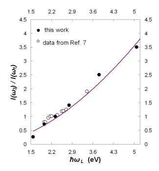
Fig. 7 - The intensity ratio of  $I(\omega_3)/I(\omega_1)$  vs. the laser excitation energy  $\hbar\omega_L$  for *trans*-(CH)<sub>x</sub> inclusions in *a*-C:H. Solid line is a theoretical calculation performed using the amplitude mode formalism [7].
