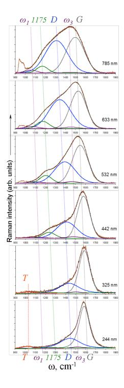
Fig. 2 - Resonant Raman spectra of *a*-C:H at 293 K showing contributions from *trans*-(CH)<sub>x</sub> ( $\omega_1$  and  $\omega_3$ ) modes, PPV (1175 cm<sup>-1</sup> mode), and DLC (*D*, *G*, and *T* modes). An asymmetric peak visible at NIR–visible (green)  $\hbar\omega_L$  at 950 cm<sup>-1</sup> is the second order *Si*, from Ref. 14.
