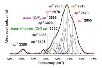
Fig. 10 - Decomposed IR stretching vibrations spectra of an *a*-C:H film. The constituent bonding groups are:  $sp^1(3300)$  *CH*,  $sp^2(3125) = C-H$  unsat/A/asym,  $sp^2(3085) = CH_2$  unsat/O/asym,  $sp^2(3050) = C-H$  sat/A/asym,  $sp^2(3020)$  trans-vinelyne (CH) sat/O/sym,  $sp^2(2995)$  trans-(CH)<sub>x</sub> sat/O/sym,  $sp^3(2970)$  -*CH*<sub>3</sub> sat/O/asym,  $sp^2(2950) = CH_2$  sat/O/asym,  $sp^3(2915) = CH$ ,  $=CH_2$  sat/O/asym,  $sp^3(2855) = CH_2$  sat/O/sym.
