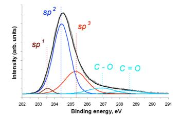
Fig. 8 - XPS core-level  $C_{1s}$  spectra of *a*-C:H; contributions for *sp*,  $sp^2$  and  $sp^3$  fractions are shown together with C-O and C=O secondary peaks.
