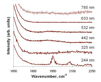
Fig. 9 - Resonant Raman spectra of sp-hybridised (polyyne) segments in a-C:H.
