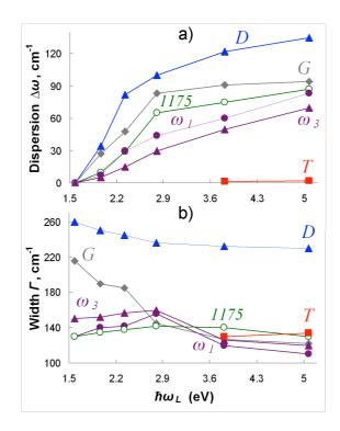
Fig. 3 a) - Peak dispersion,  $\Delta \omega$  and b) - peak widths,  $\Gamma$  for all constituent peaks as a function of the laser excitation energy  $\hbar \omega_L$ , from Ref. 14.
