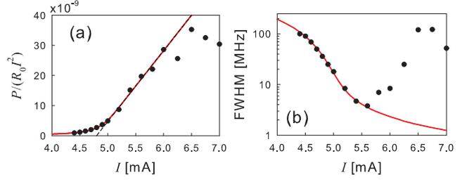
FIG. 2: (Color online) (a) Power  $P$  divided by  $R_0 I^2$  with  $R_0 = 13.6 \Omega$  and (b) linewidth (FWHM) of the signal of STNO as a function of applied current  $I$ . Dots are experimental data at  $T = 150$  K taken from Ref. 16. Red lines are theoretical fitting curves based on the model of Eq. (1).
