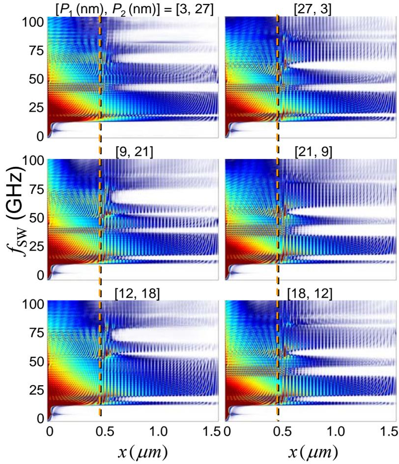
**SUPPL. FIG. 1.** Frequency spectra obtained from fast Fourier transform (FFT) of  $M_z/M_s$  oscillation along the  $x$ -axis at  $y = 15$  nm, for cases of the same  $P = 30$  nm but different  $P_1/P_2$  values as noted. The vertical dashed orange lines indicate the boundary between the single-width nanostrip waveguide (the yellow colored area in Fig. 1) and the MC of width-modulated nanostrip (the light gray colored area in Fig. 1).
