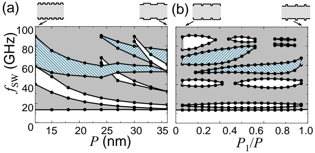
**SUPPL. FIG. 2.** Allowed and forbidden bands according to  $P$  for case of  $P_1 = P_2$  in (a) and  $P_1/P$ , maintaining  $P = P_1 + P_2 = 30$  nm in (b). The gray area indicates the allowed bands, whereas the white (blank) and blue (diagonal-line pattern) areas indicate the forbidden bands at the Brillouin zone boundary  $k = n\pi/P$ , where  $n = 0, \pm 1, \pm 2, \dots$ , and certain  $k$  values,  $k \neq n\pi/P$ , respectively.
