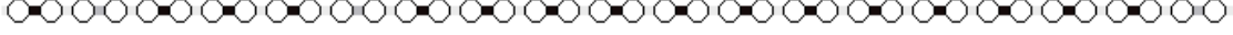
FIG. 2: (Color online) Graphical representation of a one-dimensional ring with 32 sites in the lattice structure yielding the maximal nearest-neighbor concurrence (see text). Parameters: 5000 generations; population=600. Half band filling. Three cases are distinguished by color: light grey ( |t_{ij}| < 1 ), grey ( 1 \leq |t_{ij}| < 3 ) and black ( 3 \leq |t_{ij}| < 5 ).
