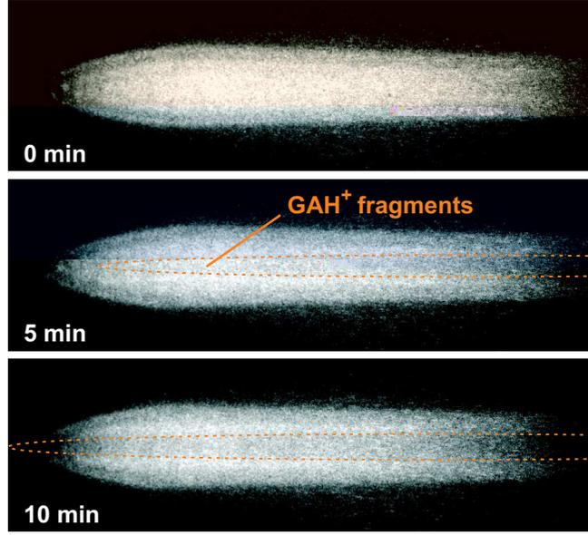
**Figure 3.** Observation of  $\text{GAH}^+$  photodestruction. An ion crystal consisting of laser-cooled  $^{138}\text{Ba}^+$  ions (visible in the CCD image), barium isotopes,  $\text{BaO}^+$  and  $\text{GAH}^+$  (all three not visible) is continuously exposed to 266 nm laser light of low intensity. The  $\text{GAH}^+$  ions dissociate within minutes, their fragments accumulate along the trap axis forming a dark core (dashed lines) inside the barium ion subensemble.
