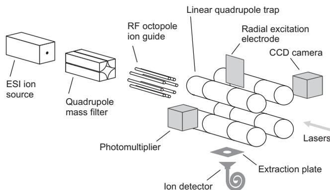
**Figure 1.** Schematic overview of the experimental setup. Protonated molecular ions from an ESI ion source are selected by a quadrupole mass filter and transferred via a RF octopole ion guide to a linear quadrupole trap in a UHV chamber. The trapped ions can be electronically excited by a radially mounted electrode and counted by an ion detector below the trap. The laser-cooled  $^{138}\text{Ba}^+$  ions are imaged with a CCD camera and their fluorescence is detected by a photomultiplier.
