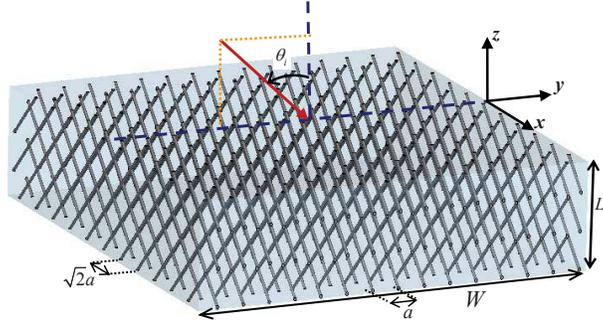
FIG. 1: (Color online) Geometry of the superlens: an array of crossed metallic wires tilted by  $\pm 45[\text{deg}]$  with respect to the interfaces is embedded in a host material slab with thickness  $L$  and relative permittivity  $\varepsilon_h$ . The wires are contained in planes parallel to the  $xoz$  plane. Each wire mesh is arranged in a square lattice with lattice constant  $a$ . The wires in adjacent planes are orthogonal, and are spaced by  $a/2$ .
