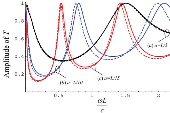
FIG. 2: (Color online) Amplitude of the transmission coefficient as a function of normalized frequency for different lattice constants,  $a$ , and a fixed slab thickness  $L$ . Solid lines: analytical model; Dashed lines: full wave simulations obtained with CST Microwave Studio [17]. The angle of incidence is  $\theta_i = 15^\circ$ , the radius of the wires is  $r_w = 0.05a$ , and the permittivity of the substrate is  $\varepsilon_h = 1$ .
