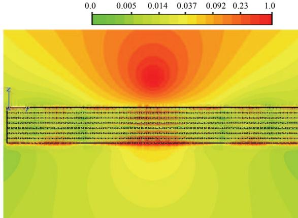
FIG. 7: (Color online) Amplitude of the normalized electric field  $E_x$  for a superlens configuration with the same geometry as case (i) of Fig. 6, except that the width of the lens along the  $y$ -direction is  $W = 0.39\lambda_0$ .
