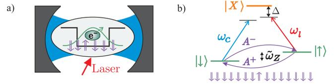
FIG. 1: (a) Singly charged QD coupled to high-Q optical cavity. (b) Level scheme of the QD. Optical and hyperfine transitions.
