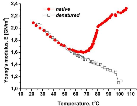
FIG. 2: Young's modulus  $E$  versus temperature for the native and heat-denatured collagen fibrils. The heating speed is 1°C/min. Red arrows and indices 1 – 5 indicate on temperature intervals discussed in the text.
