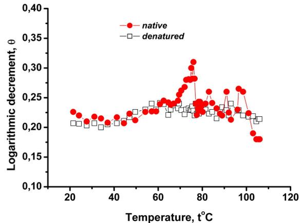
FIG. 3: The logarithmic damping decrement  $\vartheta$  versus temperature for the native and heat-denatured collagen fibrils. The heating speed is 1°C/min. The red arrow and indices 3 and 4 correspond to those in Fig. 2.
