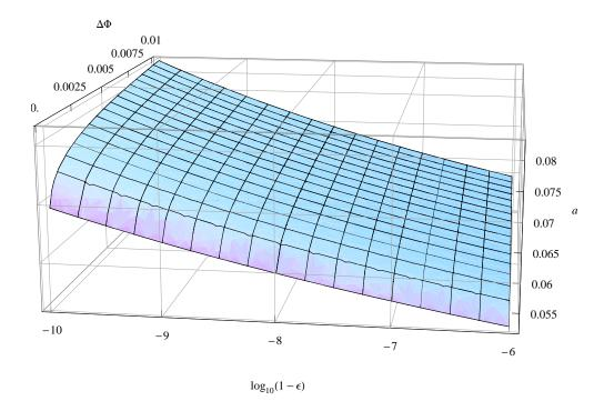
FIG. 2: Values of a (cm) for different values of  $\varepsilon$  (from 0.001 to 0.999) and  $\Delta\Phi$  (rad) (from  $10^{-4}$  to  $10^{-2}$ ) using  $^1H^+$  ion beam. The graph for the  $^{133}Cs^+$  ion beam is very similar.
