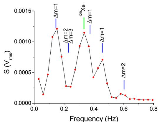
FIG. 4: A single spectrum collected with  $28 \text{ nT}$  and  $\varphi = 39^\circ$ , which corresponds to the second spectrum from the left in Fig. 3. The predicted transition frequencies are also shown for reference. The signal has the units of root-mean-squared amplitude for a  $32.768 \text{ s}$  averaging time. Given that the  $T_2$  time is about  $5 \text{ seconds}$ , we compromised on signal amplitude to achieve improved frequency resolution.
