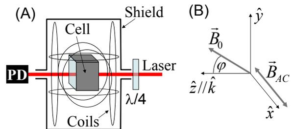
FIG. 1: (A). The apparatus. The  $1 \text{ mm}^3$  cell is roughly centered on an orthogonal three-axis set of magnetic coils. A laser beam of maximum power 3 mW enters the cell. The transmitted power is detected by a photodiode. (B). The coordinate system: the  $\hat{z}$ -axis coincides with the light propagation direction,  $\hat{k}$ . The magnetic field direction is in the  $\hat{y}$ - $\hat{z}$  plane rotated by an angle  $\varphi$  from the  $\hat{z}$ -axis.
