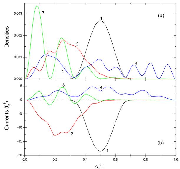
FIG. 3: (Color online.) Spatial distribution of the densities  $\rho(s, \tau)$  and currents  $J(s, \tau)$  against  $s$ . The curves "1" to "4" have  $\tau = 0, \pi/48, \pi/24,$  and  $\pi/12,$  respectively (these values are within the duration of oscillation DoS). The preset flux  $\Phi = 3.25$  (the same for Figs.3 to 6). The unit of current is  $t_o^{-1}$ , where  $t_o \equiv 2m^*L^2/(\pi^2\hbar)$  is the unit of time used in this paper.
