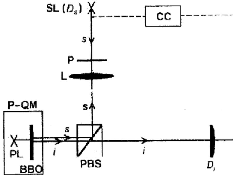
**Fig. 4:** The scheme of the experimental setup for a test of the two-photon geometric optics. The QM indicates the SPDC-quantum mirror, PBS is a polarization beam splitter, SL is a signal laser, P is an object, L a convergent lens,  $D_i$  is an idler detector and CC is the coincidence circuit
