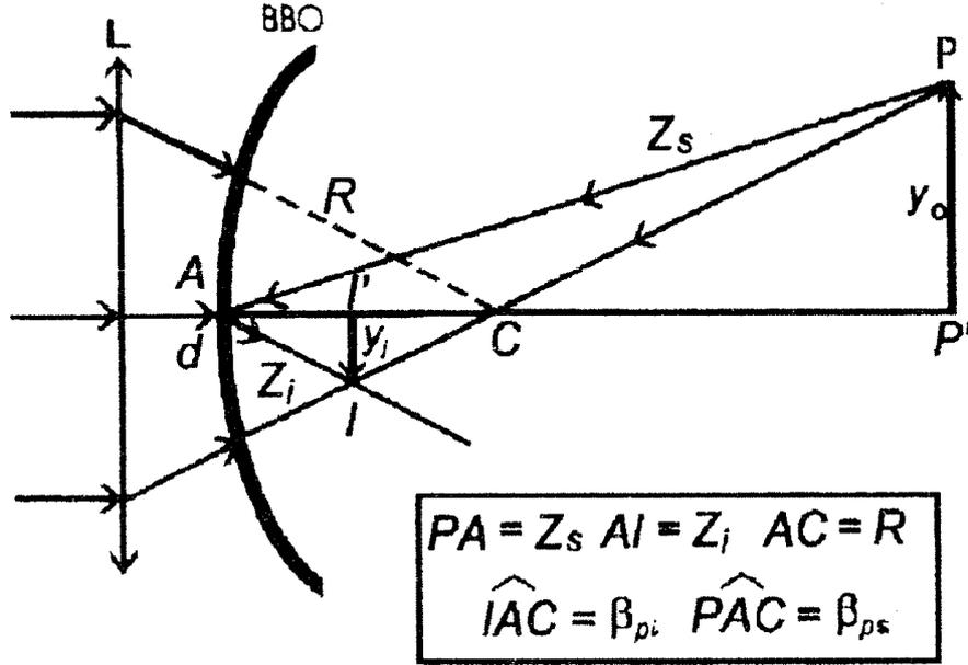
**Fig. 2b:** The basic optical configuration for a proof of magnification factor for a spherical SPDC-quantum mirror.
