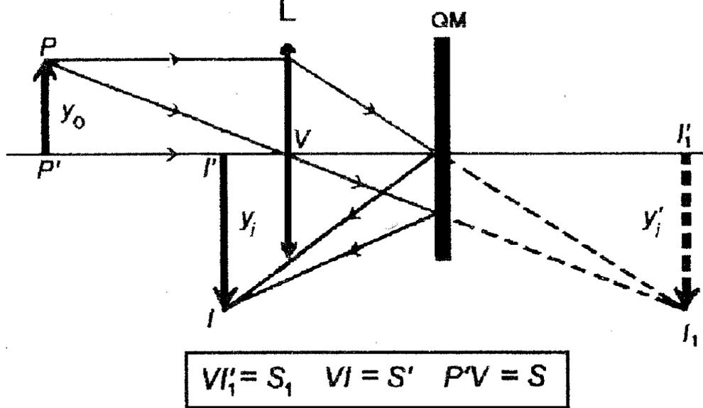
Fig. 3b: The basic optical configuration for a proof of magnification factor for a usual lens combined with a plane SPDC-quantum mirror.
