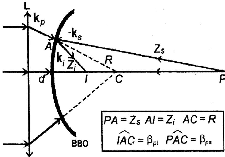
Fig. 2a: The basic optical configuration of a spherical SPDC-quantum mirror.
