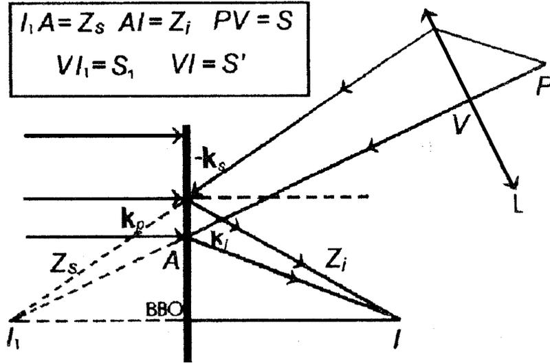
Fig. 3a: The basic optical configuration for usual lens combined with a plane SPDC-quantum mirror.
