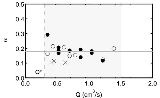
FIG. 7: **Exponent  $\alpha$  vs. flow rate  $Q$**  - The values of  $\alpha$  obtained for increasing and decreasing flow rates (respectively closed and open symbols) are almost the same and significantly smaller than  $1/2$ . Stirred samples (crosses) lead to even smaller values of  $\alpha$  (added-water content 10%,  $V = 530$  cm<sup>3</sup> and  $V = 800$  cm<sup>3</sup>,  $h_0 = 70$  mm).
