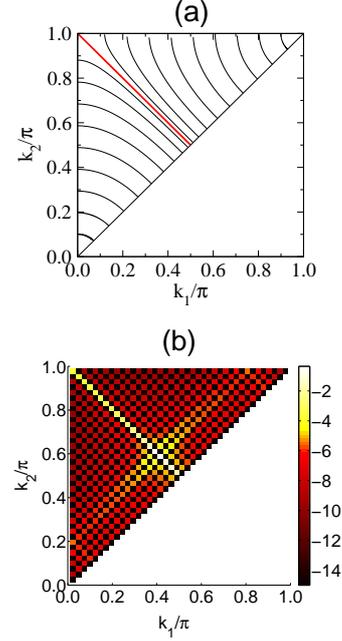
Figure 10: (a) Lines of constant energy given by (17). The red thick line is the  $E_{k_1, k_2}^0 = 0$ -line where all unperturbed states  $|k_1, k_2 = \pi - k_1\rangle$  are degenerate. (b) 3-D plot of the logarithm of the weight function in normal-mode space for the eigenstate  $\nu = 405$ , obtained by numerical diagonalization with  $\gamma = 0.1$  and  $f = 40$ . In the noninteracting case this state corresponds to  $|k_1, k_2 = \pi - k_1\rangle$ .
