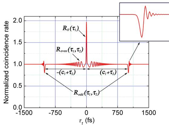
FIG. 2: The normalized coincidence rate as a function of  $\tau_1$  when a 3-mm thick ZnSe sample is placed in the MZ interferometer. The fixed delay  $\tau_2 = 26$  ps is used. The insert illustrates the odd-order dispersion contribution.
