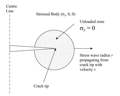
Fig. 4. Crack tip stress wave unloading model
