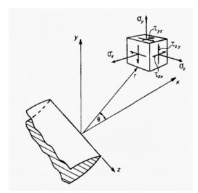
Fig. 2. Stress state at the crack tip
