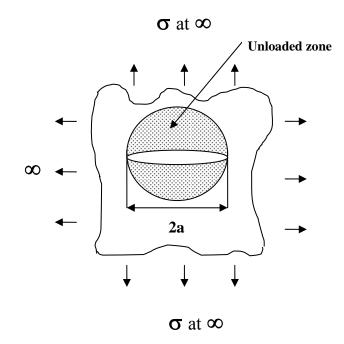
Fig. 1. The Griffith Crack
