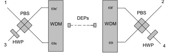
FIG. 1: The setup for bit-flip error correction in the first step. HWP and PBS represent half wave plate and polarizing beam splitter, respectively.
