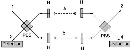
FIG. 2: The setup for the second step in our purification scheme, which is same as that in Ref.[8]. Here H and PBS represent half wave plate and polarizing beam splitter, respectively.
