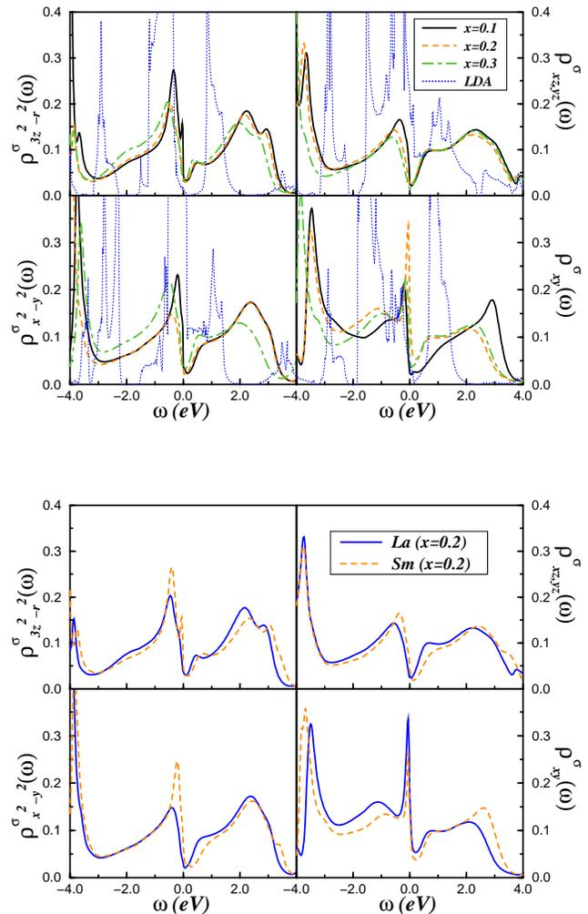
FIG. 2: (Color online) Top panel: Orbital-resolved LDA+DMFT (solid, dashed and dot-dashed) and LDA (dotted) DOS for electron-doped LaOFeAs for three doping values. The parameters are  $U = 4.0$  eV,  $U' = 2.6$  eV and  $J_H = 0.7$  eV. The drastic modification of the LDA spectra to almost totally incoherent character by large-scale dynamical spectral weight transfer is clearly visible. Bottom panel: Comparison between LDA+DMFT spectra for La- and Sm-based Fe-pnictides.
