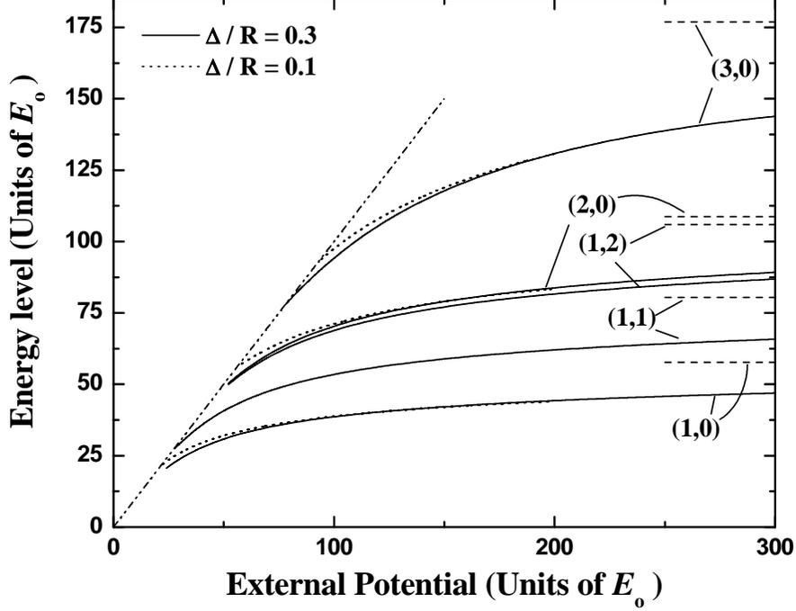
FIG. 2: First five energy levels for a lens-shaped quantum dot with  $b/a=0.51$  as a function of the external potential barrier  $\mathcal{V}_o$  in dimensionless quantities. The calculation is done taking  $\Delta/R=0.3$  (solid lines) and  $\Delta/R=0.1$  (dotted lines). In both cases it is used  $\sigma = 3.5$ . Dashed lines represent the infinite barrier case [26] while dash-dot-dot is the line where the energy value is equal to the potential value.
