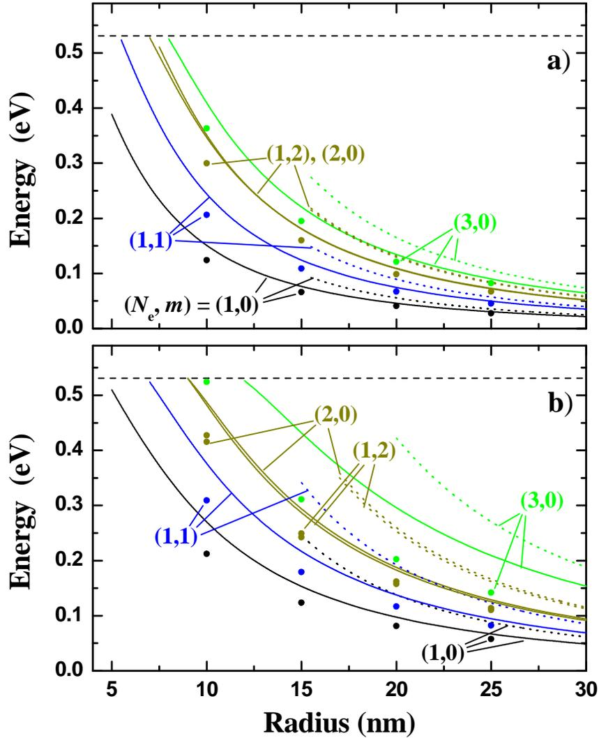
FIG. 3: First five electronic levels for an InAs/GaAs quantum lens as a function of the lens radius. a)  $b/a=0.91$ , b)  $b/a=0.51$ . The calculation is done taking  $\Delta/R=0.3$  (solid lines). Results from the infinite barrier model are also plotted for comparison (dotted lines). As a reference, the value for the confinement potential used ( $V_c = 0.531\text{eV}$ ) is shown by dashed line in both panels. Filled dots correspond to numerical calculations.
