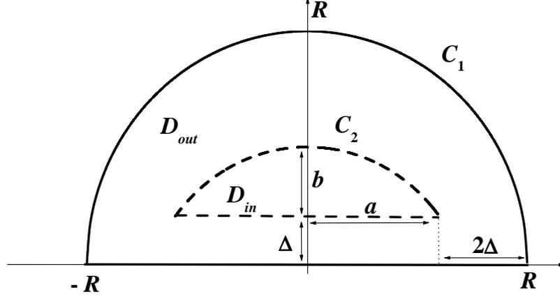
FIG. 1: Transversal section of a 3D finite lens-well  $D_{in}$  with barrier height  $V_o$  and contour  $C_2$  inside an infinite semispherical-well with contour  $C_1$ . Contour  $C_1$  and  $C_2$  are separated a distance equal or greater than  $\Delta$  along the perpendicular axis.
