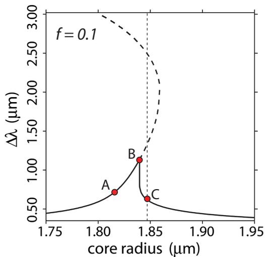
FIG. 5: (Color online) This figure is similar to Fig. 4(a), for the case  $f = 0.1$ . Here we have used a larger plotting range to better represent the branch of the generated bandwidth vs radius curve corresponding to the satellite peaks. The spectra associated with points A, B and C are discussed in Sec. IV.
