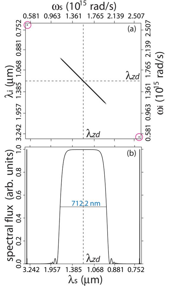
FIG. 7: (Color online) (a) Representation of the joint spectral intensity in  $\{\omega_s, \omega_i\}$  space, for the same parameters as in Fig. 6. Note that there are two highly non-degenerate satellite peaks, shown circled. (b) Singles spectrum corresponding to the joint spectral intensity in (a).
