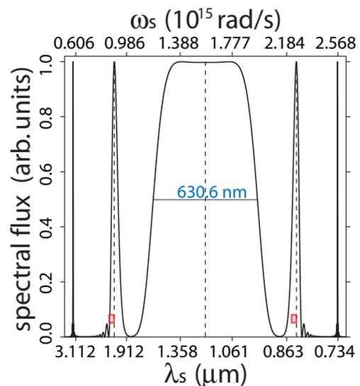
FIG. 9: (Color online) Singles spectrum corresponding to point C in Fig. 5. The red rectangles represent the  $\sim 40$  THz spontaneous Raman scattering bandwidth centered at the inner NDP frequency pair.
