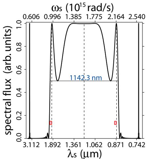
FIG. 8: (Color online) Singles spectrum corresponding to point B in Fig. 5. The red rectangles represent the  $\sim 40$  THz spontaneous Raman scattering bandwidth centered at the inner NDP frequency pair.
