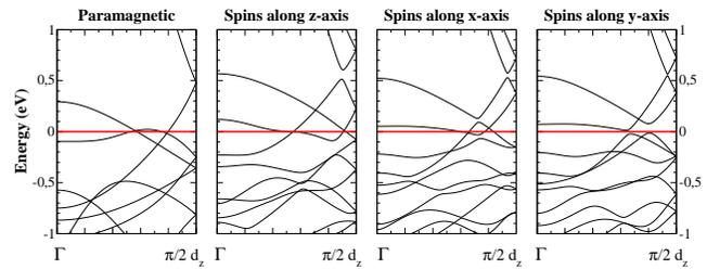
FIG. 4: Band structure of a zigzag platinum chain with an elongation  $d_z = 2.45$  Å. From left to right the panels show the bands for a paramagnetic calculation, and for spin-orbit simulations whereby the spins are oriented along the  $z$ -,  $x$ - and  $y$ -axes, respectively.
