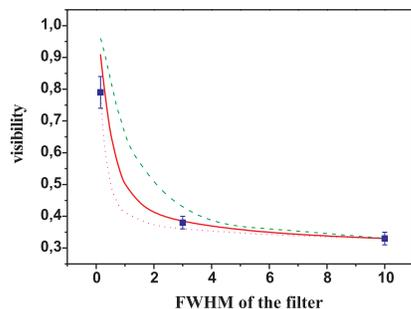
FIG. 5: Interference visibility measured (points) and calculated (solid line), as a function of the filter bandwidth. Dashed line shows the same dependence calculated for the case of a two-photon state twice less entangled (TPSA twice as broad) and dotted line, for the case of a state twice more entangled (TPSA half as broad).
