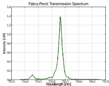
FIG. 4: Transmission spectrum of a FP with 300  $\mu\text{m}$  base. The central peak corresponds to the degeneracy point, the side one is due to its imperfect suppression by two IFs
