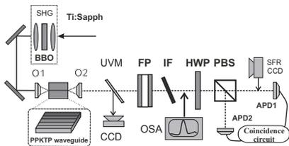
FIG. 2: Experimental setup. Second harmonic of Ti:Sa laser radiation is focused into a 12 mm type-II PPKTP waveguide, where SPDC is produced; O1 and O2 are the coupling/decoupling objectives; UVM, highly reflective UV mirror; HWP, half-wave plate; PBS, polarizing beamsplitter; APD1, APD2, single-photon counting modules; FP, Fabry-Perot interferometer; OSA, optical spectrum analyzer; IF, interference filters; SPR CCD, single-photon resolving CCD camera combined with a grating spectrometer.
