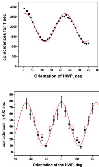
FIG. 3: Experimental dependencies of the coincidence counting rate on the HWP orientation for (a) 3 nm filtering and (b) 0.15 nm filtering. Solid lines represent a fit of experimental data.
