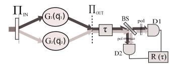
FIG. 1: Scheme of the proposed setup. Horizontally-polarized photons from type-II SPDC are assigned a phase dependent on the photon transverse momentum  $\phi_o(q_o)$ , while the vertically-polarized ones are assigned a phase  $\phi_e(q_e)$ . The modulated photons enter a type-II quantum interferometer, which records the coincidence count rate as a function of the delay  $\tau$  between the photons given by an appropriate delay-line.
