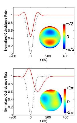
FIG. 5: Examples of the shape of the polarization quantum-interference dip with two different spatial phase modulations (in black the unperturbed dip, in red the modulated one). In the upper figure the effect of a small amount of coma along the vertical axis is shown. In the lower figure a more complicated superposition of aberrations affects dramatically the shape of the dip
