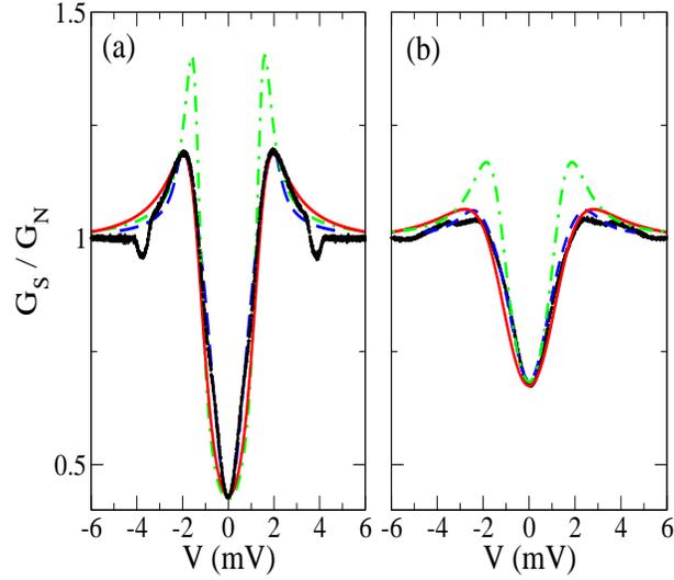
**Figure 2.** Normalized tunneling conductance of junction 2 measured at  $T = 1.5$  K (a) and  $3.945$  K (b), together with a fit to Models I (dash-dotted green), II (dashed blue) and III (solid red).
