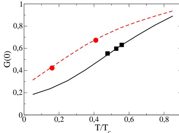
**Figure 5.** Zero-voltage conductance  $G(0)$  as a function of reduced temperature. Red circles and black squares correspond to the experimental data of J2 and J3, respectively. Dashed red and solid black lines correspond to the values of  $G(0)$  obtained with Model III, using the parameters shown in Table II.
