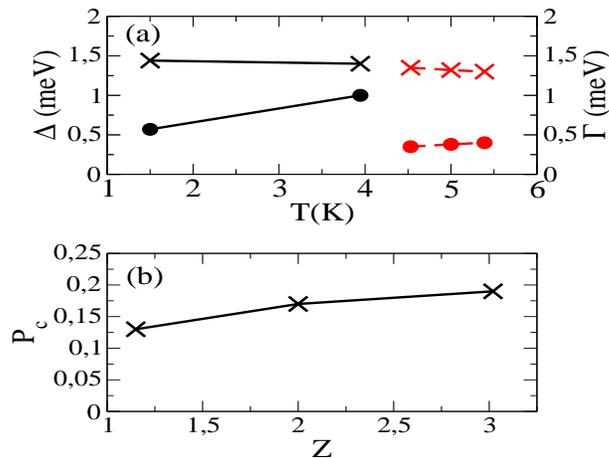
**Figure 6.** (a) Values of the superconducting gap (crosses) and the Dynes parameter (circles) as a function of temperature obtained from the fits of our Generalized BTK model to the normalized conductance of junctions 2 (black) and 3 (red). (b) Current polarization as a function of the height  $Z$  of the delta-function barrier entering our Generalized BTK model for the three junctions studied in this article. Lines have been added to aid the eye.
