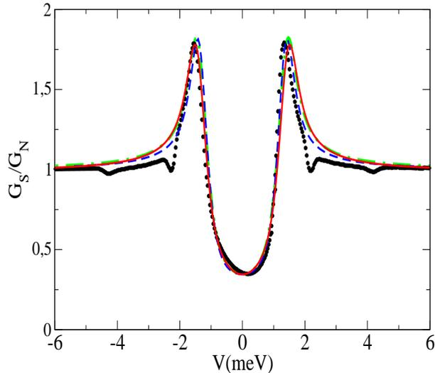
**Figure 1.** Normalized tunneling conductance of junction 1 measured at  $T = 1.52$  K. Black circles indicate experimental data; dashed-dotted green lines are fits to Model I, dashed blue, fits to Model II, and solid red, fits to Model III.
