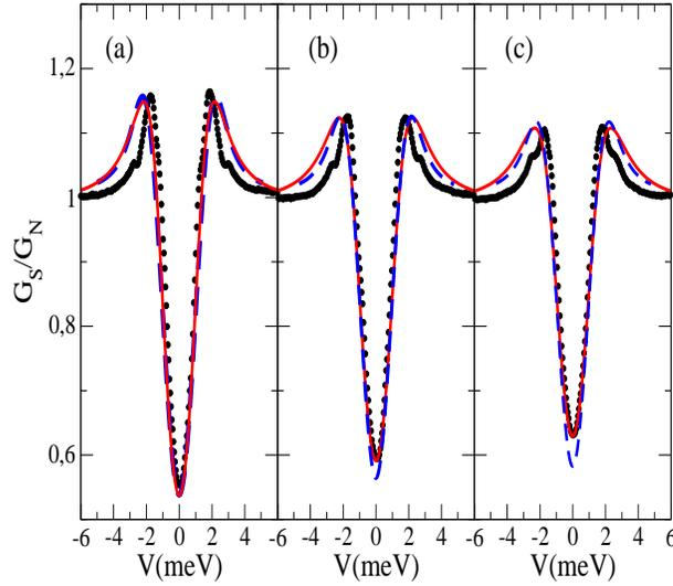
**Figure 3.** Normalized tunneling conductance of junction 3 measured at  $T = 4.53$  K (a),  $5.0$  K (b) and  $5.39$  K (c), together with a fit to Models II (dashed blue) and III (solid red).
