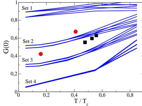
**Figure 4.** Zero-voltage conductance  $G(0)$  as a function of reduced temperature. Red circles and black squares correspond to the data of J2 and J3, respectively. Sets 1, 2, 3 and 4 correspond to  $T_{av} = 0.15, 0.4, 0.55$  and  $0.7$ , respectively. Each set has 6 lines, that correspond to the different combinations of  $P_c = 0.15$  and  $0.35$ , and  $\Gamma = 0.1, 0.3$  and  $0.5$ .
