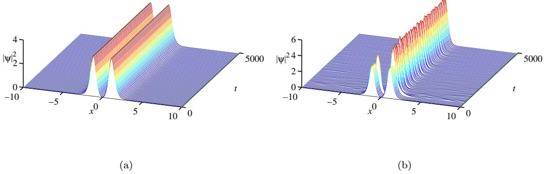
FIG. 7: (Color online) (a) An example of a stable antisymmetric state with  $a = 1$ , for  $\mu = -1.3$  and  $N = 6.7137$ . (b) The evolution of an unstable antisymmetric state, also with  $a = 1$ , but for  $\mu = -1.5$  and  $N = 7.1273$ .
