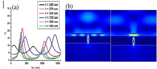
FIG. 4. (Color online) (a) Dependence of the transmission efficiency on the width of the metallic nano-strip for different nano slit thicknesses with  $H_p=50nm$ ,  $d=44nm$ ,  $W_s=25nm$ ; (b) Distributions of magnetic field  $|H_y|$  for (left)  $t=240nm$  and  $W_p=1410nm$  or (right)  $t=300nm$  and  $W_p=360nm$ .
