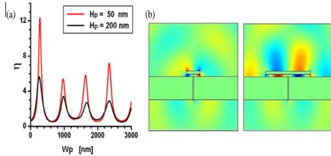
FIG. 3. (Color online) (a) Dependence of the transmission on the width of the metallic nano-strip for different nano-strip heights with  $W_s=25nm$ ,  $t=390nm$  and  $d=44nm$ ; (b) Distributions of electric field  $E_z$  for (left)  $W_p=280nm$  (right) or  $970nm$  when  $H_p=50nm$ .
