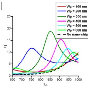
FIG. 5. (Color online) Transmission spectrum for various metallic nano-strip widths when  $t=240nm$  (the dashed line is for the corresponding bare nano slit).  $H_p=50nm$ ,  $d=44nm$ ,  $W_s=25nm$ .
