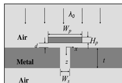
FIG. 1. Configuration of the nano cavity antenna formed by a nearby metallic nano-strip over the opening of a nano slit milled in a metallic thin film.
