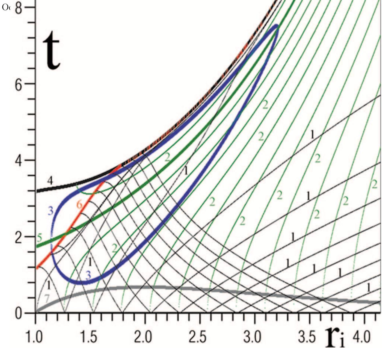
Figure 1: Diagrams  $t(r_i/q)$ : 1 - for light geodesics; 2 - for  $r = \text{const}$ ; 3 - for the apparent horizon and the inner horizon; 4 - for the limiting stopping time; 5 - for the throat  $r = q$ ; 6 - for the intersection times of adjacent dust layers; 7 - the dependence  $s(r_i/q) = 0.7(r_i/q - 1) \cdot \exp(2 - r_i/q)$  — the scale for  $s$  (vertical axis) coincides with the time scale  $t$ .
