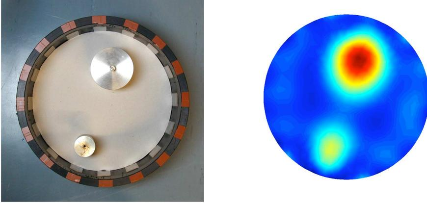
Figure 4: **Left:** An EIT measurement configuration for imaging objects in a tank. The electrodes used for measurements are at the boundary of the tank, which is filled with a conductive liquid. **Right:** A reconstruction of the conductivity inside the tank obtained using boundary measurements. [Jari Kaipio, Univ. of Kuopio, Finland; by permission.]
