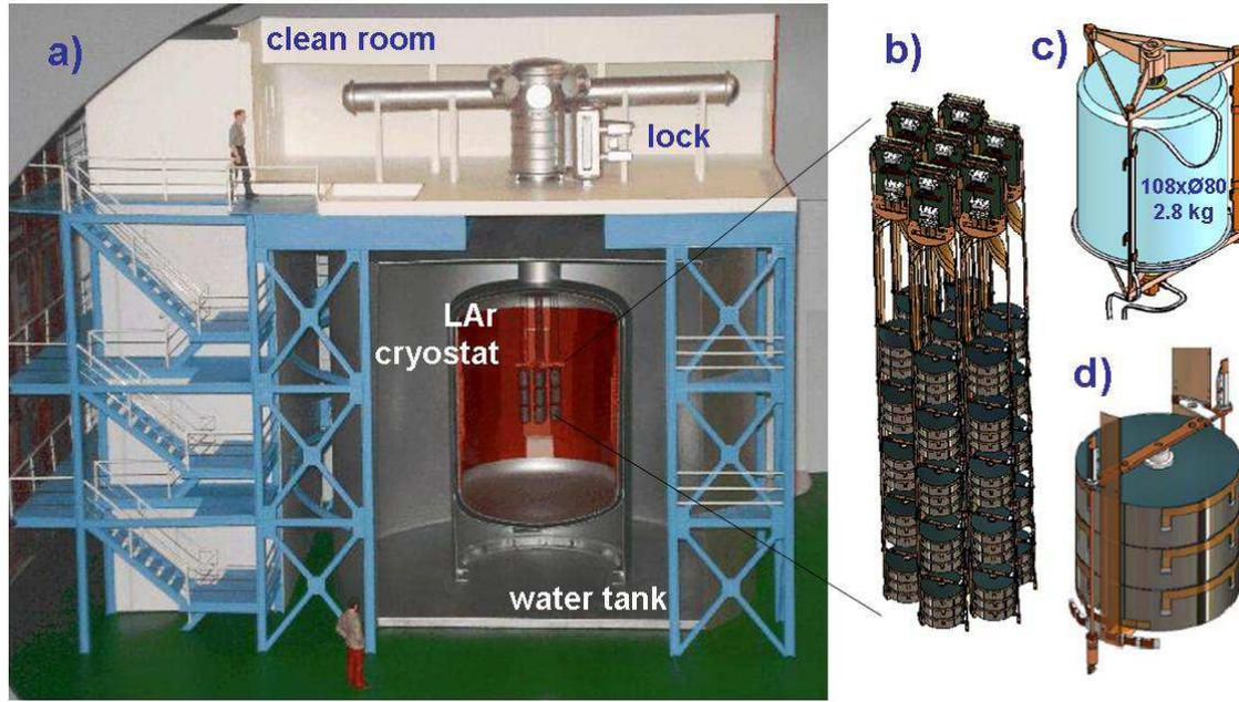
Figure 1: Artist's views of a) the GERDA experiment, b) a  $5 \times 7$  Ge detector array assembled from 7 strings of 5 diodes, c) a p-type Ge diode for phase I and d) a segmented true coaxial n-type Ge diode for phase II in low mass support and contact structures. Laboratory rooms behind the staircase are allocated for the water plant and a radon monitor (ground floor), a control room (first floor), and for vacuum, cryogenic and electronic components (second floor).
