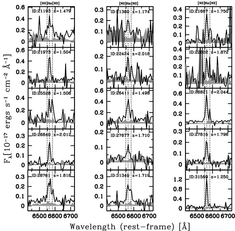
Fig. 2.— The spectra of H $\alpha$  and [N II] emission lines we have detected. These spectra have a binned dispersion of  $\sim 16$   $\text{\AA}$ . The solid lines show the spectra and the shaded regions in gray are the  $1\sigma$  sky noise. We regard lines with a peak flux larger than the  $3\sigma$  sky noise as a detection using unbinned 1D spectra. Labeled redshifts are derived from H $\alpha$  lines.
