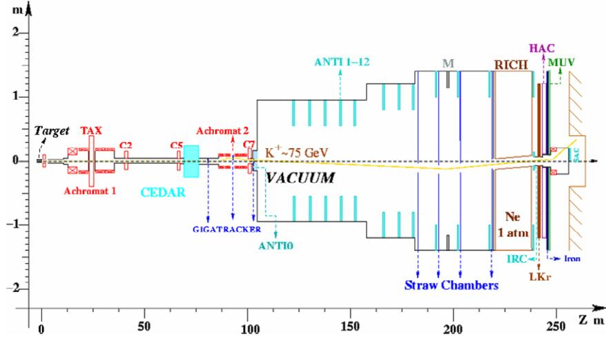
Figure 1: Layout of the NA62 experiment
